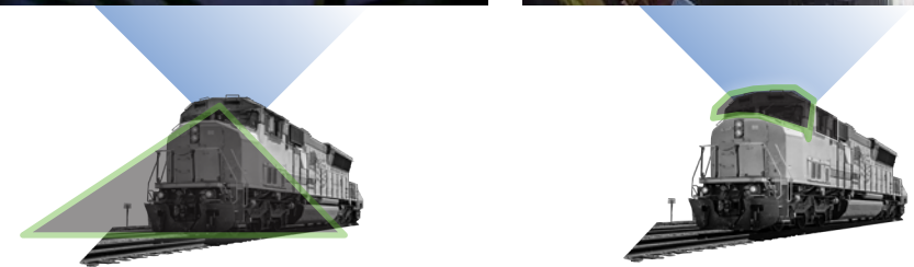
A forward-facing camera captures conditions in front of the locomotive and two in-cab dome cameras that monitor all activity in the cab.
