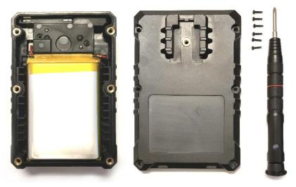
4. Remove the original battery from the camera and set it to the left of the camera so the wires are accessible.
