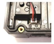
6. Connect the new battery to the white connector in the upper left of the camera, ensure the red wire is oriented towards the top as designated.
