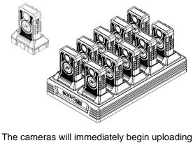
once connected. The camera display will show the upload status. Always check the display before removing a camera from the dock; do not remove if a firmware update is in progress.
